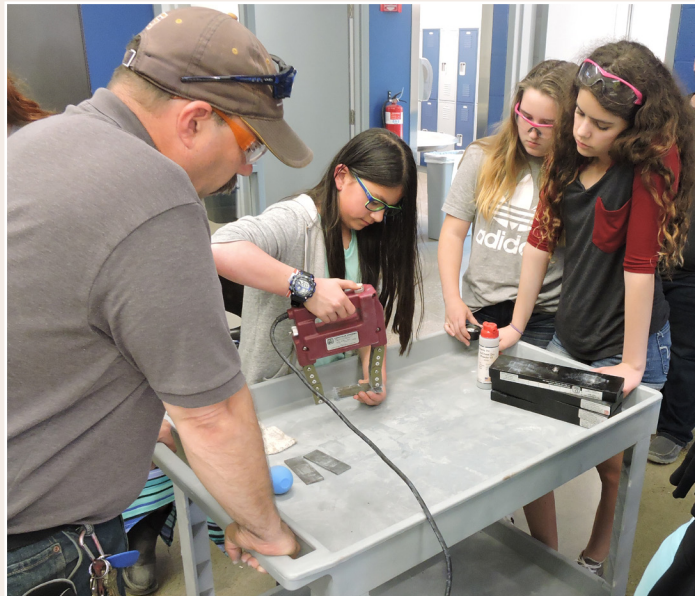
Scott Ballard oversees Pipeline participants as they use a yoke tester to perform a magnetic particle test on a sample of steel. This test is part of the Non-destructive Testing degree to ensure high-quality parts for planes, rocket and satellite parts.
